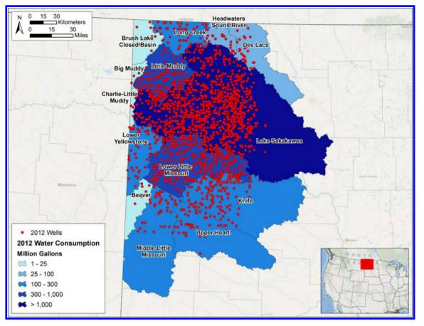
Figure 1. 2012 Hydraulic Fracturing Locations and Water Use by HUC-8 Subbasin in the North Dakota Bakken Shale Play. This figure overlays well installations in 2012 upon the estimated water use for hydraulically fracturing those wells, summed by HUC-8 watershed subbasin.
