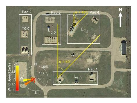
**SM\_Figure 5.** An example of weak-interference scenario during Week-1 of testing at **METEC.** The 10-minute binary yes/no detection test scenario had a 2 m/s average wind from 202.6° and leaks on pads 1 and 4. Because pad 4 could experience potential interference from pad 1, the results from pad 4 were discarded from statistical analysis. Here, the 40° cone contained 80% of all wind vectors in the 10-minute test period.
