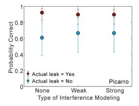
**SM\_Figure 8. Interference analysis of Picarro Inc.'s performance.** The fraction of correctly identified tests for true positives (red), and true negatives (blue) across the three scenarios considered in this analysis. The error bars correspond to 95% confidence intervals associated with finite sample sizes.
