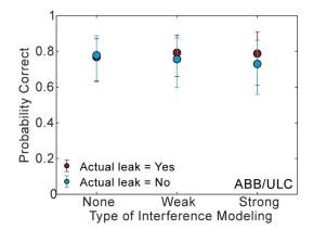
**SM\_Figure 13. Interference analysis of ABB/ULC Robotics' performance.** The fraction of correctly identified tests for true positives (red), and true negatives (blue) across the three scenarios considered in this analysis. The error bars correspond to 95% confidence intervals associated with finite sample sizes.
