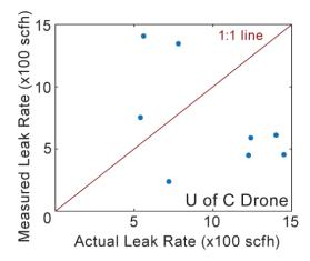
SM\_Figure 3. Performance results of University of Calgary (drone) in the Stanford/EDF Mobile Monitoring Challenge. Quantification parity chart between actual and measured leak rates. The drone technology was tested only on one of the days due to airspace restrictions resulting in a small sample size.
