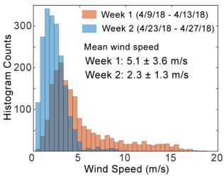
254 SM Figure 4. Wind speed distribution at METEC during the S
