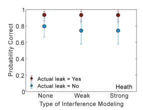
**SM\_Figure 7. Interference analysis of Heath Consultants' performance.** The fraction of correctly identified tests for true positives (red), and true negatives (blue) across the three scenarios considered in this analysis. The error bars correspond to 95% confidence intervals associated with finite sample sizes.
