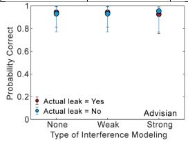
**SM\_Figure 12. Interference analysis of Advisian's performance.** The fraction of correctly identified tests for true positives (red), and true negatives (blue) across the three scenarios considered in this analysis. The error bars correspond to 95% confidence intervals associated with finite sample sizes.
