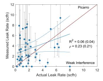
**SM\_Figure 9: Quantification parity chart for Picarro under the weak- and strong-interference scenarios.** While there was marginal improvement in R<sup>2</sup>, the average error also increased from -0.9 scfh to -1.3 scfh. The parameter values in parenthesis represent base-case scenario.
